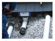
All Center and Side Track Pans are molded with pipe fitting locators at their lowest point. Below-grade piping can be installed to channel large spills to oil/water separators, holding ponds, etc.
